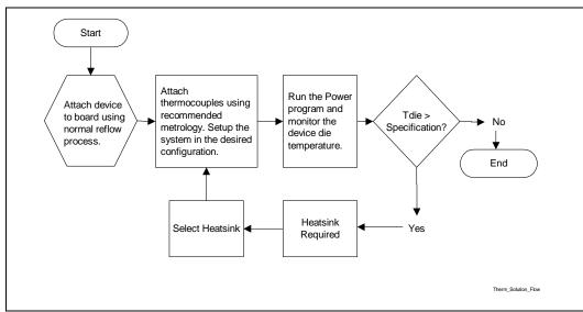
Figure 5-2. Zero Degree Angle Attach Methodology
